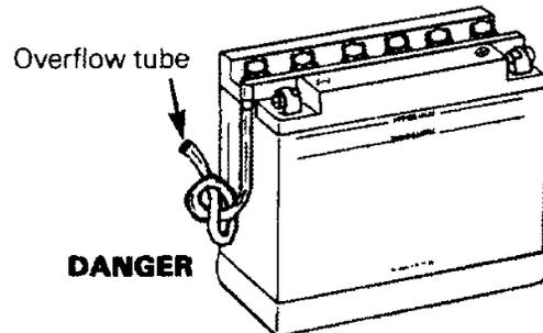
**CAUTION:** Prior to charging the battery, always remove it from the vehicle to prevent electrolyte spillage.
