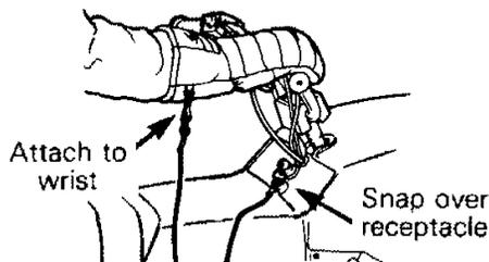
If emergency engine "shut off" is required completely pull cap from safety switch and engine power will be automatically shut "off".
