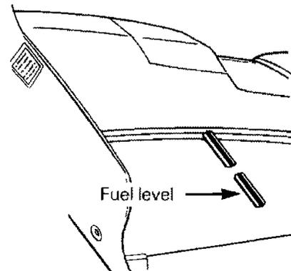
◆ **WARNING:** Never use a lite match or open flame to check fuel level.
