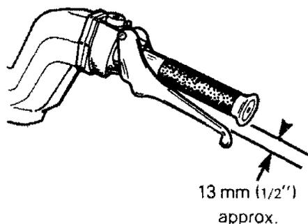
The brake mechanism is a self-adjusting type. If a quicker brake response is desired, strongly pull the brake lever several times, this will actuate the self adjusting mechanism.
