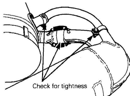
On fan cooled models, ensure that the forced flow system is well aligned and tightened.
