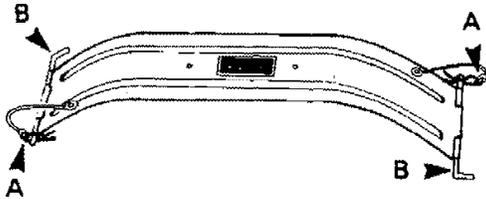
◆ **WARNING:** At the removal or installation of the belt guard front retaining pin be careful not to burn yourself on the exhaust system.
