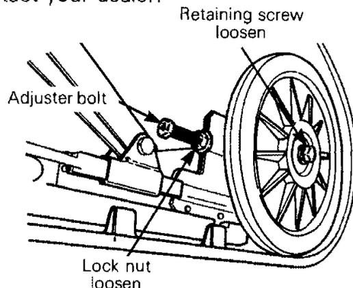
○ **NOTE:** Track tension and alignment are inter-related. Do not adjust one without the other.
