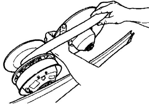
4. Slip the belt out from the drive pulley and remove completely from the vehicle. To install the drive belt, reverse the procedure.
