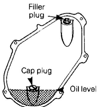
The oil should be level with the bottom of the oil level orifice.
