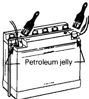
Check that battery is well secured and that battery overflow tube is not blocked or kinked.
