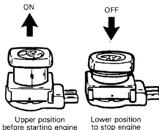
The driver of this vehicle should familiarize himself with the function of this device by using it several times on first outing. Thereby being mentally prepared for emergency situations requiring its use.
