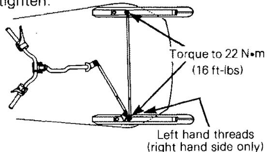
▼ **CAUTION:** Do not overtighten the left hand threaded ball joint jam nut.
