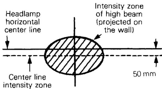
To adjust, remove headlamp chrome ring, turn upper or lower adjusting screws to obtain desired beam position.
