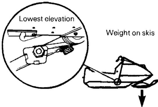
At the highest position the weight is transferred from the skis to the track. The rear adjuster blocks should be adjusted to suit the driver's preference.
