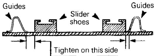
Tighten lock nuts and recheck the alignment. Ensure to retighten the idler wheel retaining screws.
