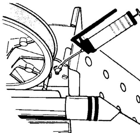
▼ **CAUTION:** When lubricating the drive axle bearing, do not apply excessive grease as the seal will be pushed out of its housing. Check seal position with finger.
