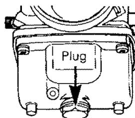
Re-install plug and connect fuel line. Check all fuel lines, replace if necessary.
