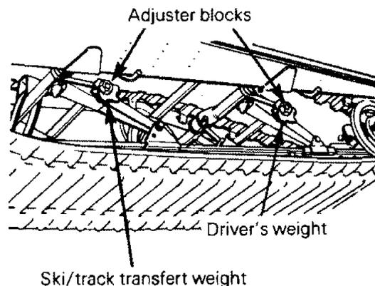
When the front adjuster blocks are at the lowest elevation more weight is distributed on the skis.
